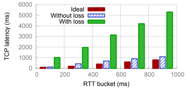
Figure 1: Mean TCP latency to transfer an HTTP response from Web server to a client. Measurements are bucketed by packet round-trip time between the frontend and the client.
